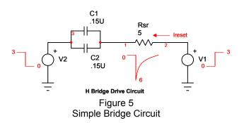
From the figure, sources V1 and V2 are combinations of charged capacitors and transistor switches that are timed to change voltage levels at the same moment, creating a double supply voltage swing across C1, C2, and the set/reset strap resistance (Rsr). Since the capacitors can not suddenly change their voltage, all of the voltage change is across Rsr until C1 and C2 begin to store a charge. With 3 volts as the supply, then 6 volts is theoretically available for the strap.
